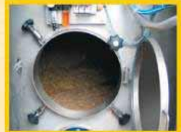
A rich, oxygenated slurry is produced and held within the tank until full.
